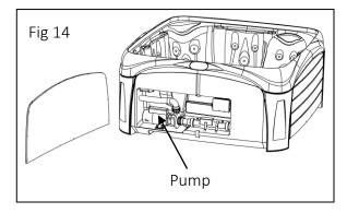
The pipes entering and leaving the pump are connected with large plastic unions. To purge the air from the pump, one of these unions will be slightly loosened.
