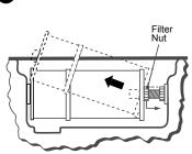
Loosen filter nut to provide clearance, then remove filter assembly.
