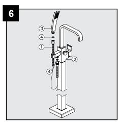
Connect one end of the shower hose (1) to the mixer (2) and the other end to the hand shower (3). Ensure the washer (4) is in each end for seal.
