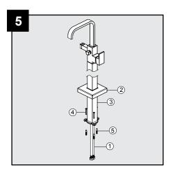
Place the assembly with the flexible supply lines (1) through the prepared hole and then holding the escutcheon (2), secure the standpipe (3).
