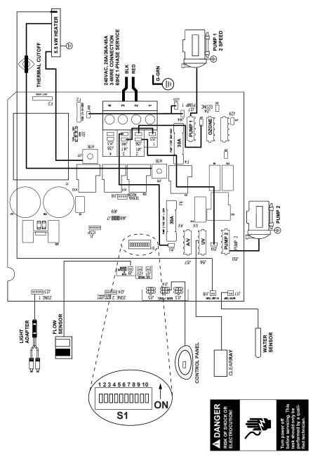
**16.2** North American J-115<sup>™</sup> and J-125<sup>™</sup> Convertible Models This wiring diagram is used for the 120/240V 60 Hz North American convertible spa models.
