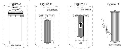
To ensure optimum performance, clean skimmer basket and filter cartridge once a month or as necessary, depending on use.
