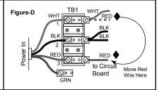
North American Convertible Models: 120 VAC, 3-Wire Connection 60 Hz North American Convertible Models: 240 VAC, 4-Wire Connection 60 Hz
